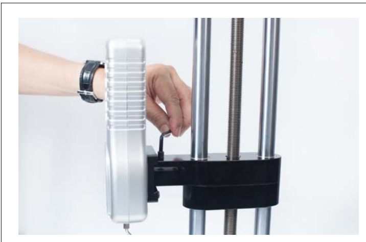
Use the 4 mm hexagonal spanner ( 2-3 , Fig. 2 )
