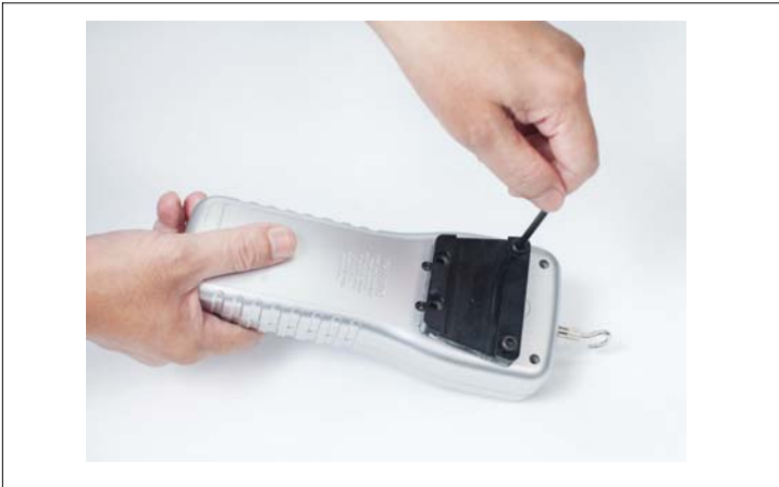
Use the 4 mm hexagonal spanner ( 2-2 , Fig. 2 )
