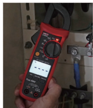
NCV multi-segment display and audio/visual alarm
