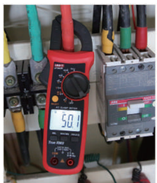
High voltage (600V) frequency measurement
