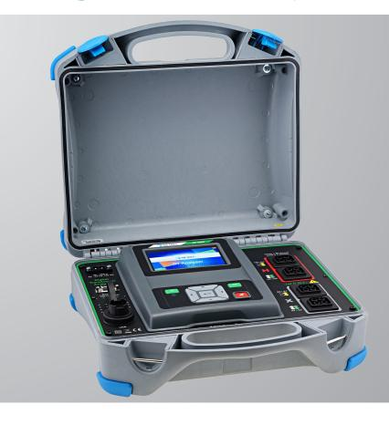
Digital Transformer Analyser (MI 3280) is a Multi-function, portable battery (Li-ion) powered test instrument with excellent IP protection: IP65 (case closed), IP54 (case open), intended for diagnosing of: turn ratio, phase deviation and excitation current of single and three phase transformers and winding resistance of single and three phase transformers.
