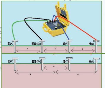
Wenner method: the distances between the 4 rods are identical:  $d_0W = 2.\pi.d.R_{SSE}$
