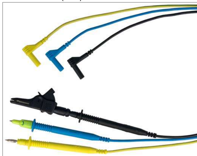
Measurement cables (black, blue, yellow-green) with test probe and safety caps (CAT IV 300 V, CAT III 600 V), as well as alligator clips (CAT III 1000 V)
